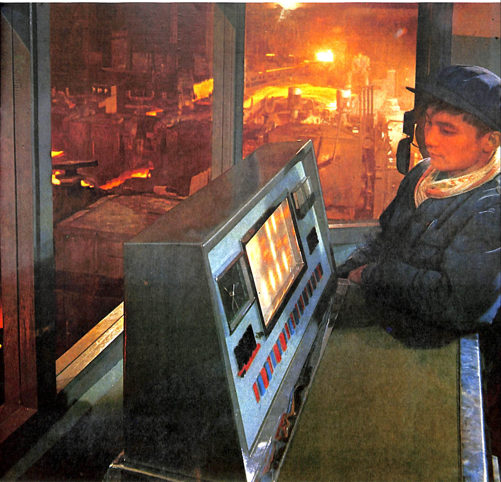
Simple program-control equipment automates the production of hot-rolled band steel at the Changchow Steel Works.
